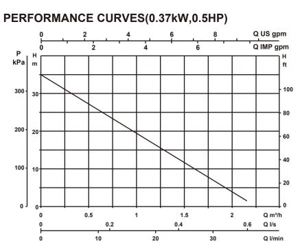
The performance curves are based on the kinematic viscosity values = 1 mm<sup>2</sup>/s and density equal to 1000 kg/m<sup>3</sup>. Curve tolerance according to ISO 9906.
