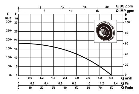
The performance curves are based on the kinematic viscosity values = 1 mm²/s and density equal to 1000 kg/m³. Curve tolerance according to ISO 9906.
