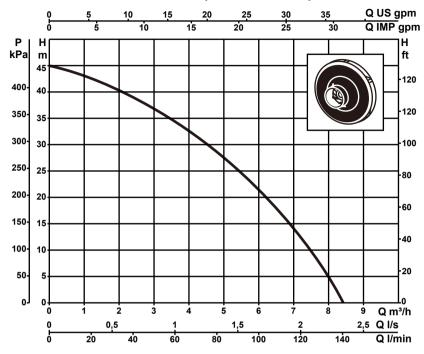
The performance curves are based on the kinematic viscosity values = 1 mm²/s and density equal to 1000 kg/m³. Curve tolerance according to ISO 9906.
