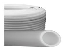
All 5-layer PE-RT pipes from MAINCOR are oxygen tight according to DIN 4726 due to the embedded EVOH layer. Thanks to the unique molecular structure a crosslinking is not necessary to achieve long term stability. During the Coextrusion all layers are being produced simultaneously; therfore a homogeneous and very stable material bonding is created.
