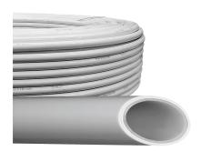
MAINCOR multilayer composite pipes are made of overlapped welded aluminium surrounded by PE-RT layers connected by adhesives.
